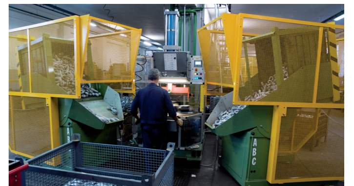
Vibration dampers automatic assembly line
