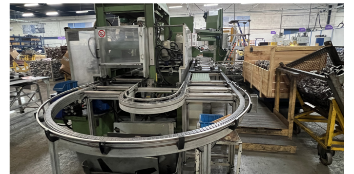
Spacer dampers automatic assembly line
